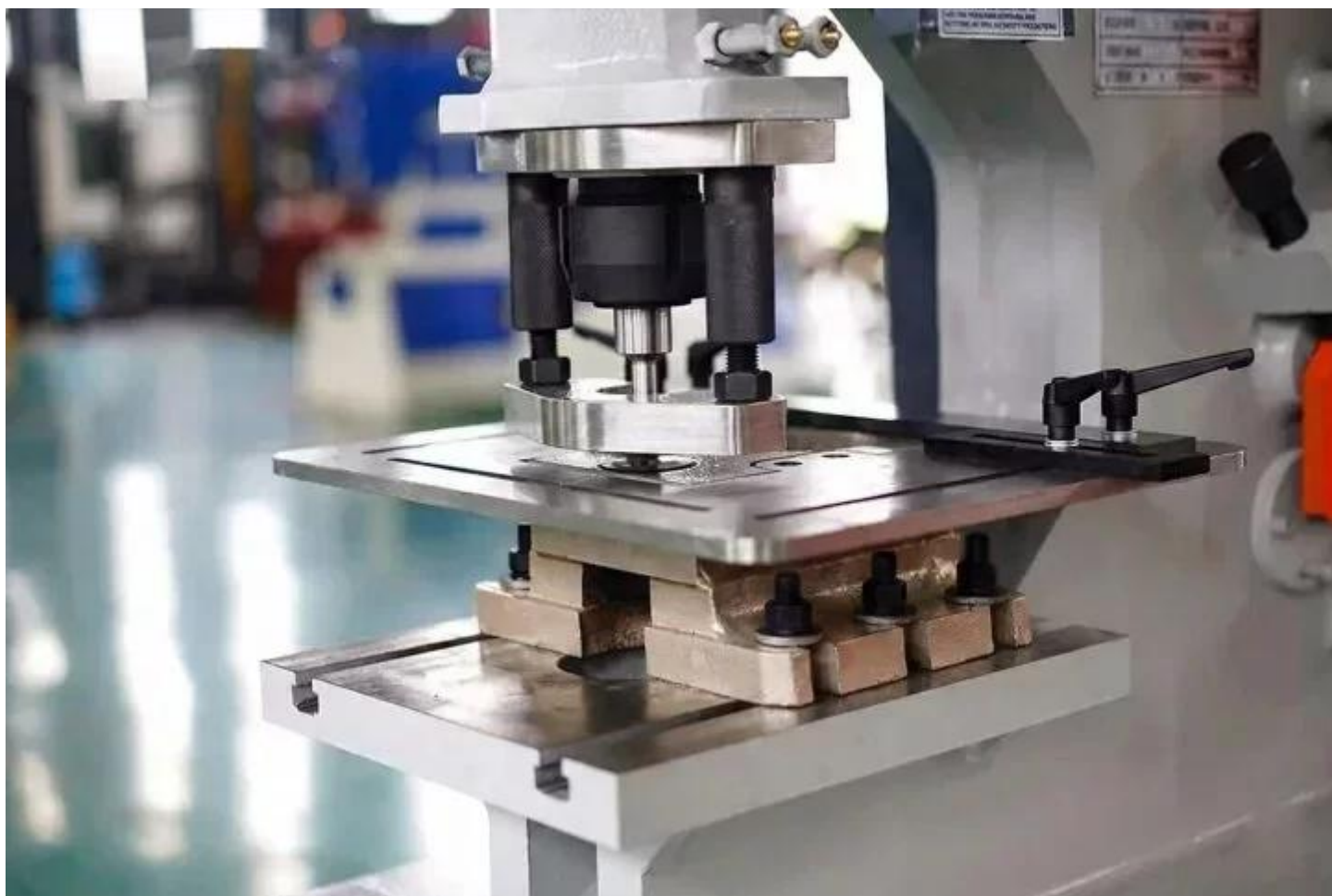
Punching station — 60-ton pressing force
